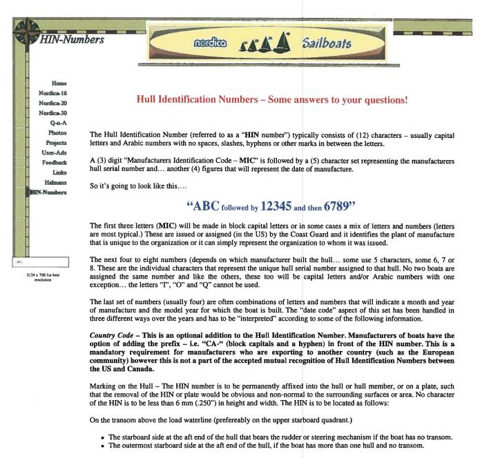
Some manufacturers had added some additional characters after the HIN but separated from the HIN by a hyphen. (Keep in mind this system is geared to work with all boats, pleasure, commercial, aluminum, fiberglass, sail, power, etc. – so the hull and manufacturer variations do take in some latitude.)
